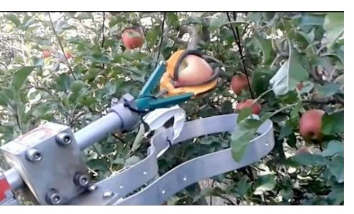
**Example: FFRobotics' Apple Picking Robot** mimics human hand movements to carefully detach apples from trees.
