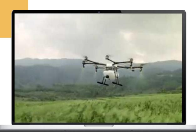
**Example:** DJI Agras MG-1 drone autonomously sprays crops 40 times faster than manual spraying, ensuring even coverage and reducing water usage.
